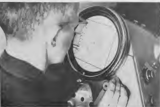
AN ESSO Research scientist examines a hydrocarbon sample on the screen of an electron microscope. The scale, right, is in microns. The electron microscope permits over 100,000 fold magnification up to 100,000 fold. UN CIENTISTA di Esso Research ta examina un muestra di hidrocarburo arriba pantalla di un microscopio electrónico. E escala, abao, ta den microns. E sorto di microscopio aki ta permiti magnificacian te 100,000 vez.
